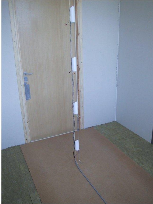
Figure 3.4. The strings on which the shielded air temperature sensors are mounted.
