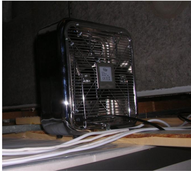
Figure 3.21. Fan for circulating the air above the test room.
