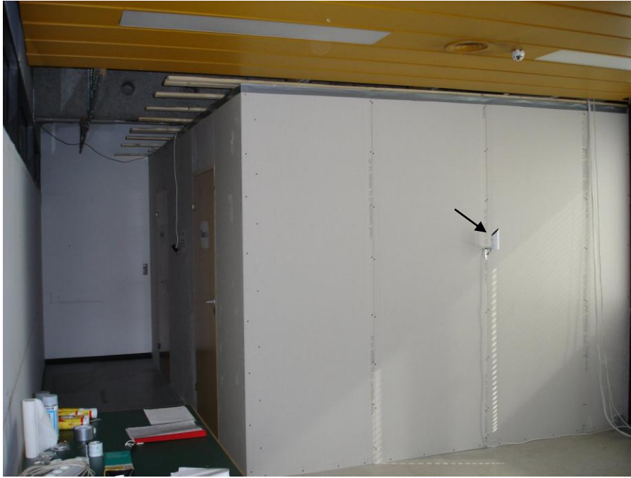
Figure 3.8. The shielded air temperature sensor in the laboratory to the West of the test rooms.
