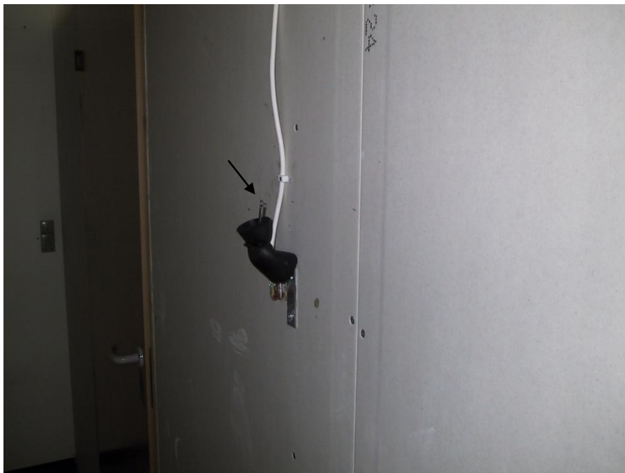
Figure 3.9. The air temperature sensor in the laboratory to the North of the test rooms.
