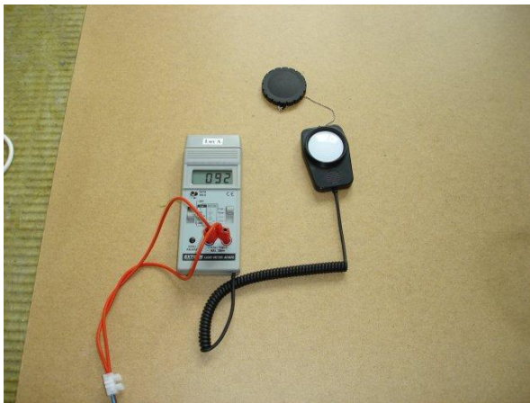
Figure 3.17. One of the two luxmeters. At the top installed on a adjustable and movable tripod. Bottom to the left: the instrument and bottom to the right the plane of the tripod with levels to insure horizontal location of the sensor.
