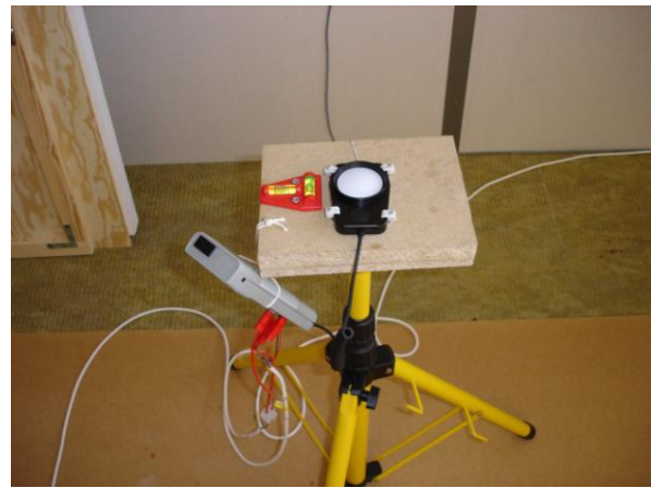
Figure 3.17. One of the two luxmeters. At the top installed on a adjustable and movable tripod. Bottom to the left: the instrument and bottom to the right the plane of the tripod with levels to insure horizontal location of the sensor.
