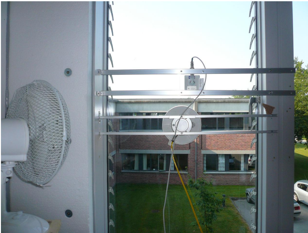
Figure 4.11. The arrangement for testing the measurements of incoming solar radiation through the traditional low-E window.
