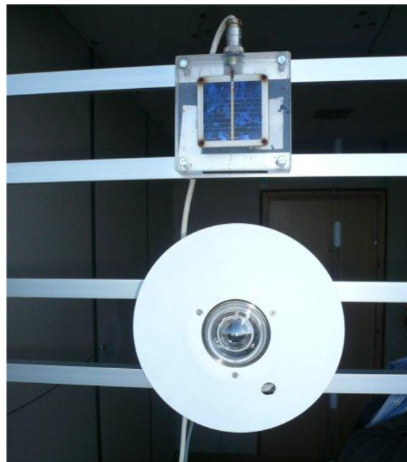
Figure 3.1. The Epply pyranometer applied for measuring the solar radiation through the MicroShade window in test room A. The Epply pyranometer is shown together with the original pc-pyranometer which turned out to be less applicable for measuring solar radiation through MicroShades due to a too low measuring band width – it cannot measure solar radiation above 2000 nm.
