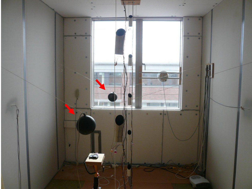
Figure 7.6. Globe temperature sensors in test room B.
