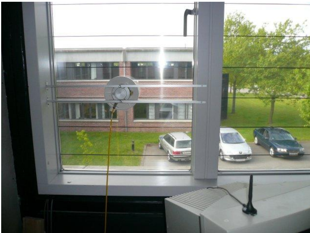
Figure 1.2. A photo through a window with MicroShades. MicroShades are manufactured in a role to role production. The width of the foil is 140 mm. The vertical stripes in figure is 3 mm opaque areas for mounting of the MicroShades.
