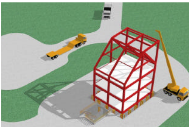
Figure 1. Components of the steel skeleton of the test facility.
