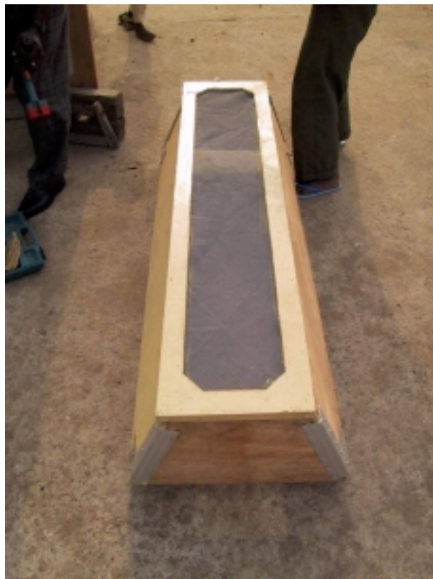
Figure 5. The extension box of the drying bed.
