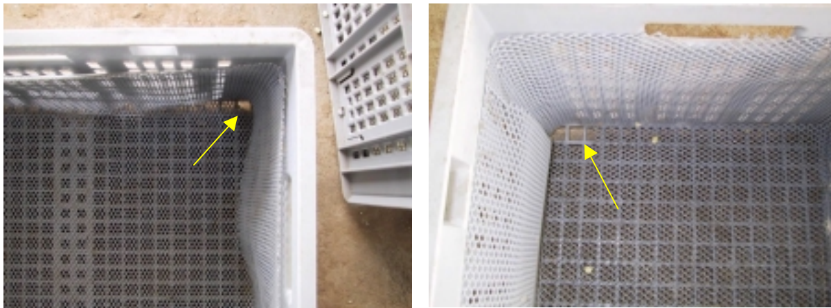
Figure 9. Two drying trays with a hole in the corner of the net in the bottom of the trays.
