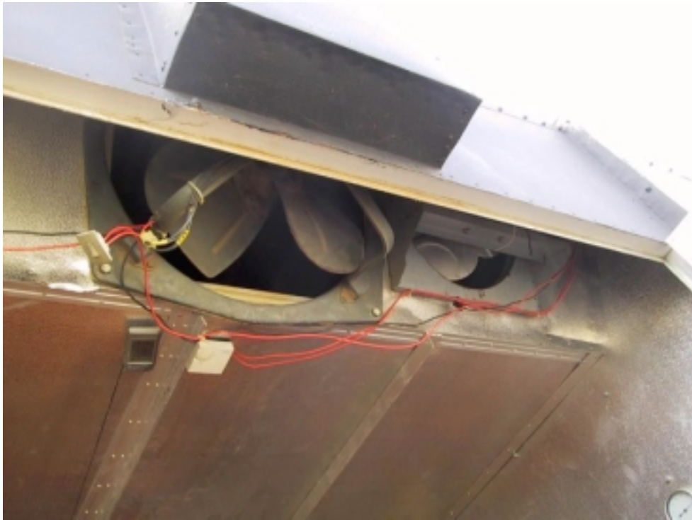
Figure 6. The fans of the solar kiln.
