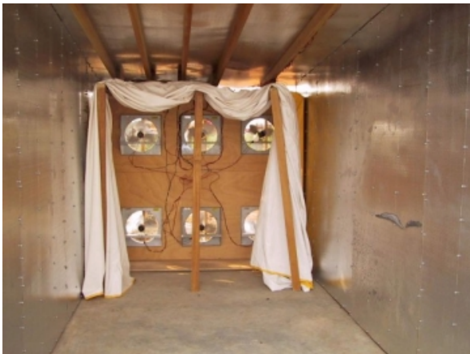
Figure 2. The pressure chamber of the forced open air dryer with fans and the tarpaulin.
