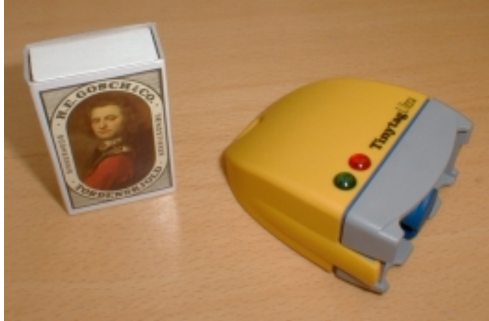
Figure 5. Picture of a Tinytag for combined measuring of the air temperature and the air relative humidity together with a Danish matchbox.
