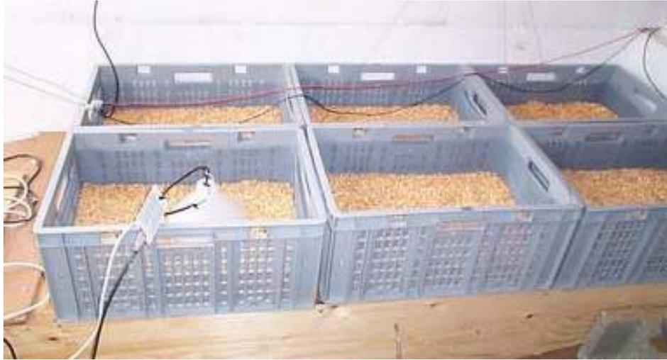
Figure 3.4. The new drying trays made of plastic.
