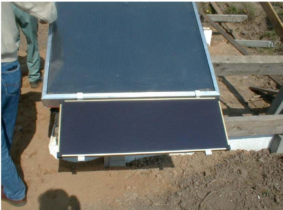
Figure 2.9. The bottom PV-panels of the dryer.
