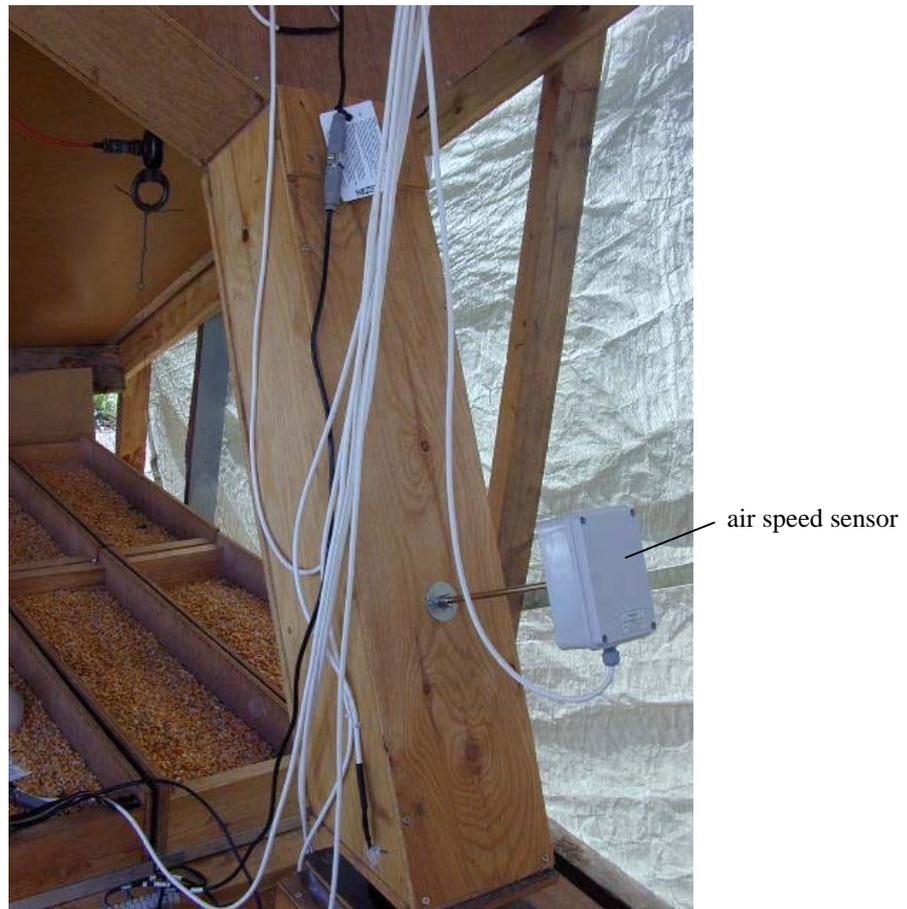
Figure 2.18. The air speed sensor.
