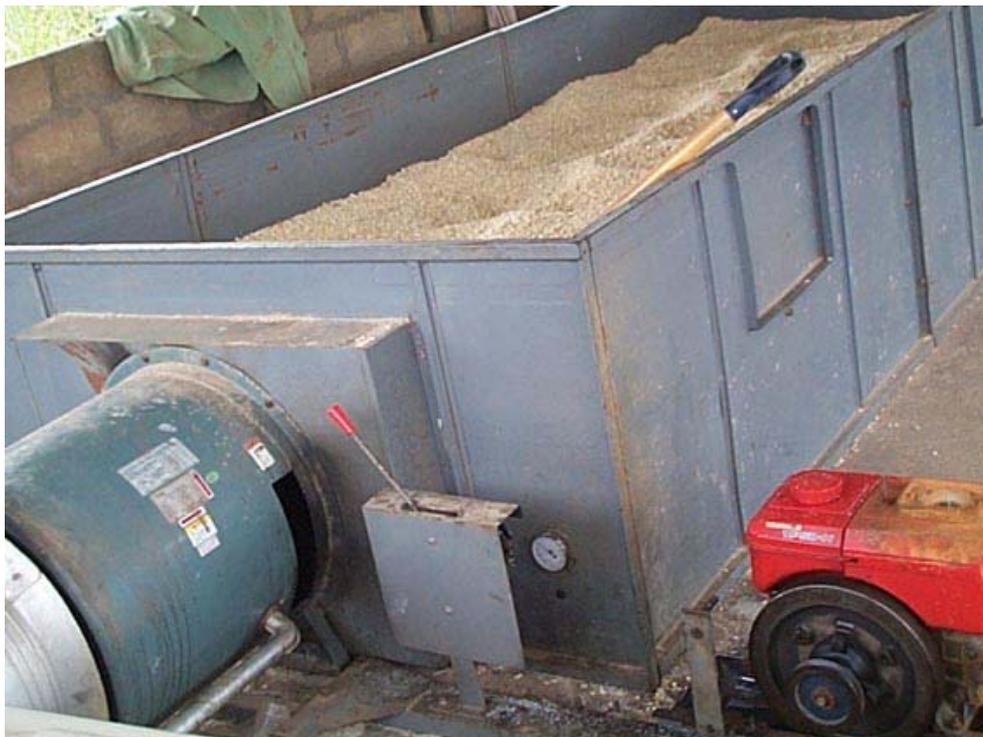
Figure 7.1. The batch dryer at Silwood Farms used for drying of maize
