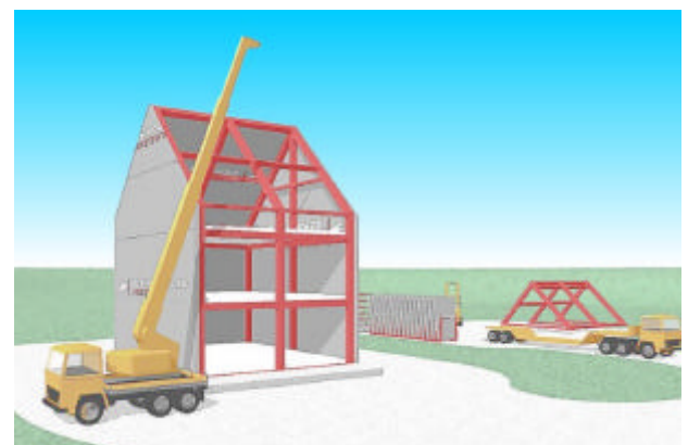
Figure 3. The test facility in its maximum configuration with adiabatic panels on all facades.
