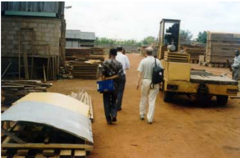
Photo 15: Mobile covering for timber
