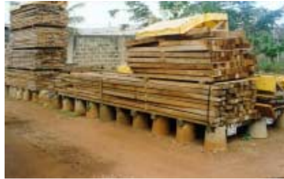
Photo 17: Far too small sticker dimension will result in too poor ventilation through the stacks
