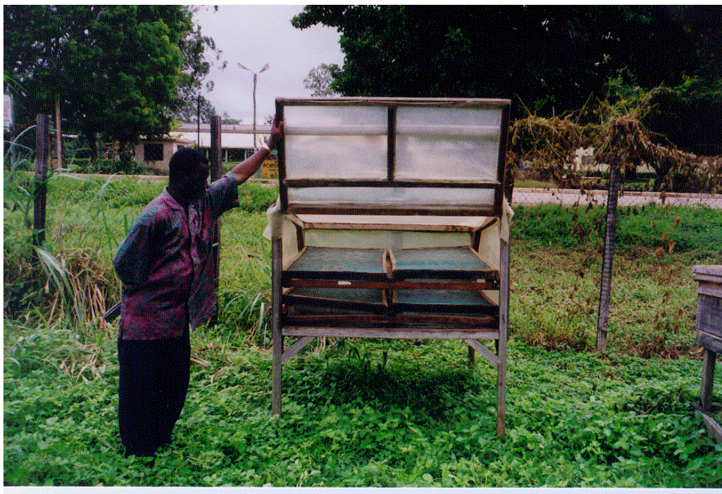
Figure 2.4. Cabinet dryer with 4 drying trays
