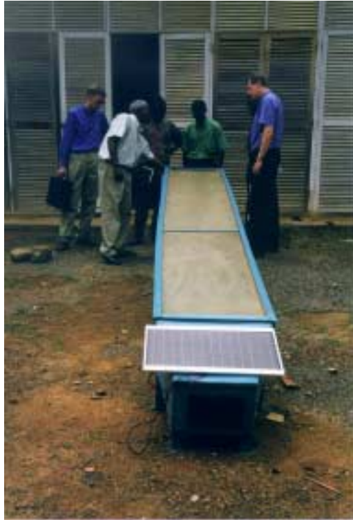
Figure 5.4. Small fan driven solar air collector.
