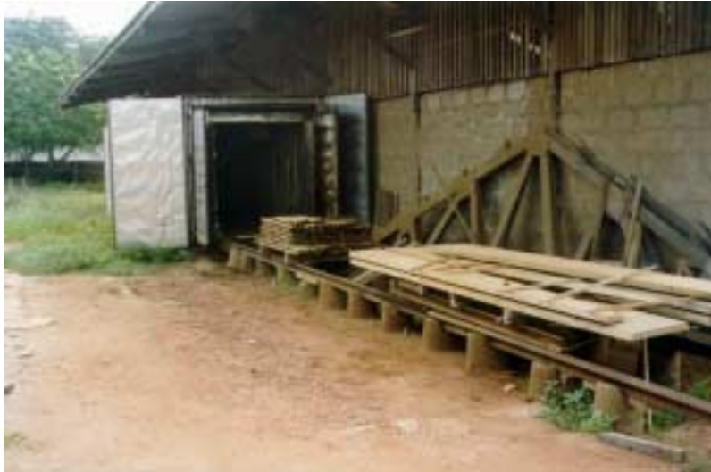
Photo 14: Container rebuilt into a drying kiln
