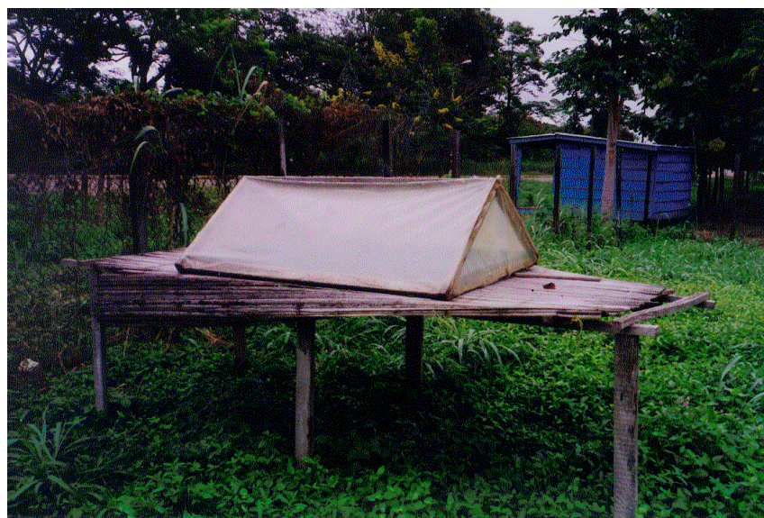
Figure 2.3. Improved drying table. Traditional drying tray covered with a simple solar collector made from timber and polythene sheet.
