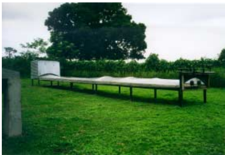
Figure 5.6. Ghanaian dryer - type K - based on the principle in the German dryer.
