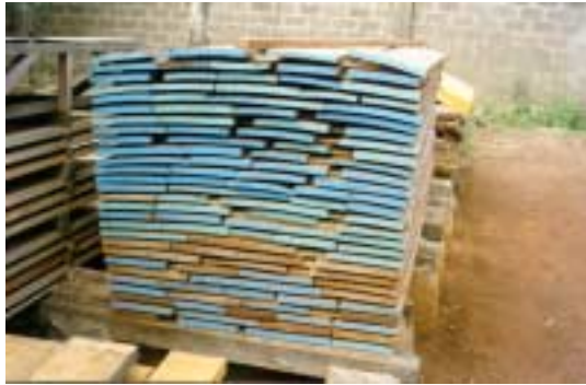
Photo 16: Stack of timber with deformations
