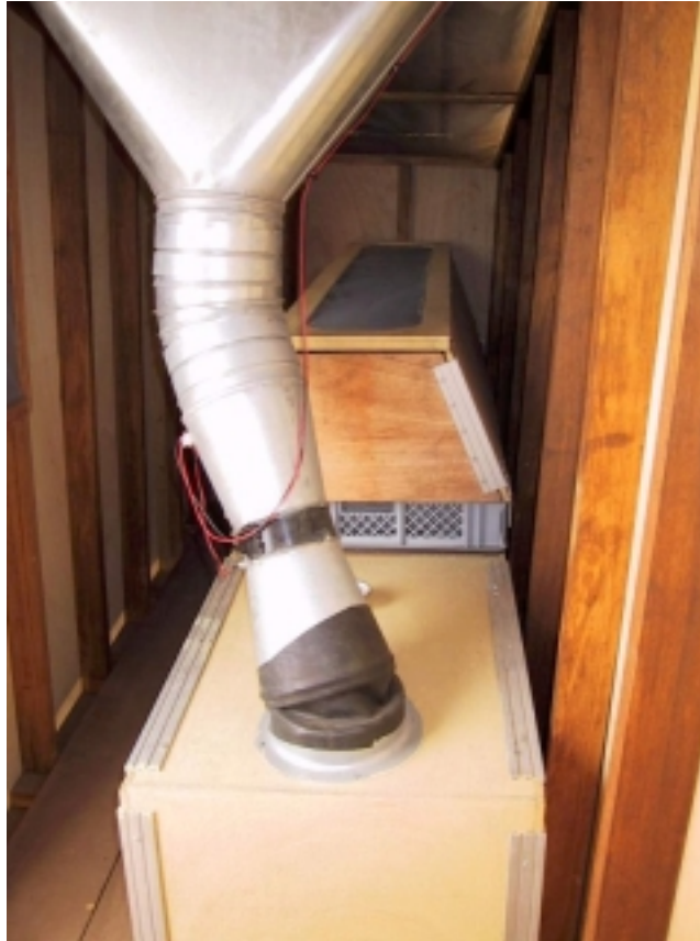
Figure 6.4. The interior of the hut containing the drying bed of the solar fish dryer.
