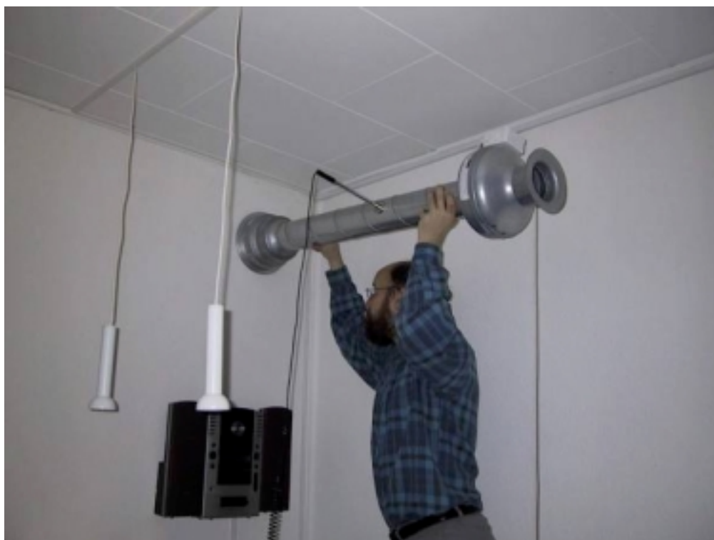
Figure 2.8. Calibration of the air speed sensors in the inlet from the PV-gable.
