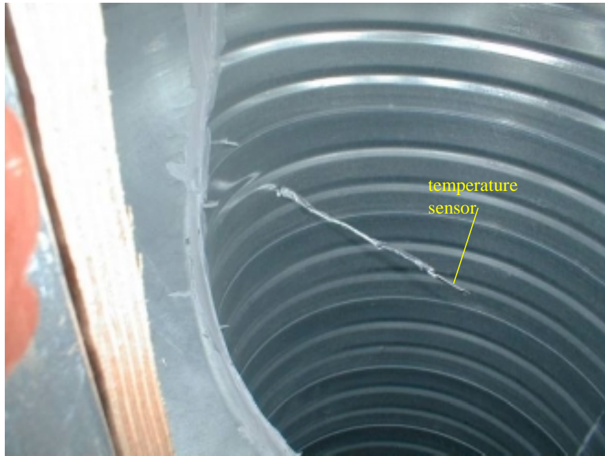
Figure 2.21. Example of the location of an air temperature sensor in the outlet of a solar ventilation chimney.
