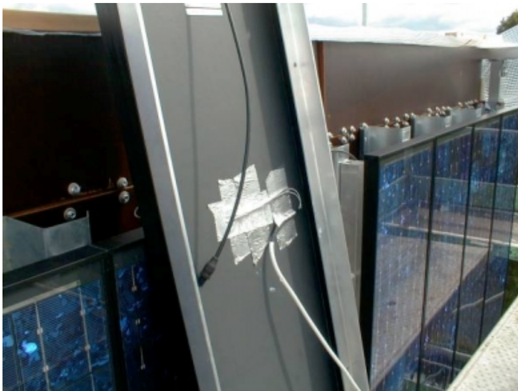
Figure 2.18. A surface sensor mounted at the back of a PV-panel.
