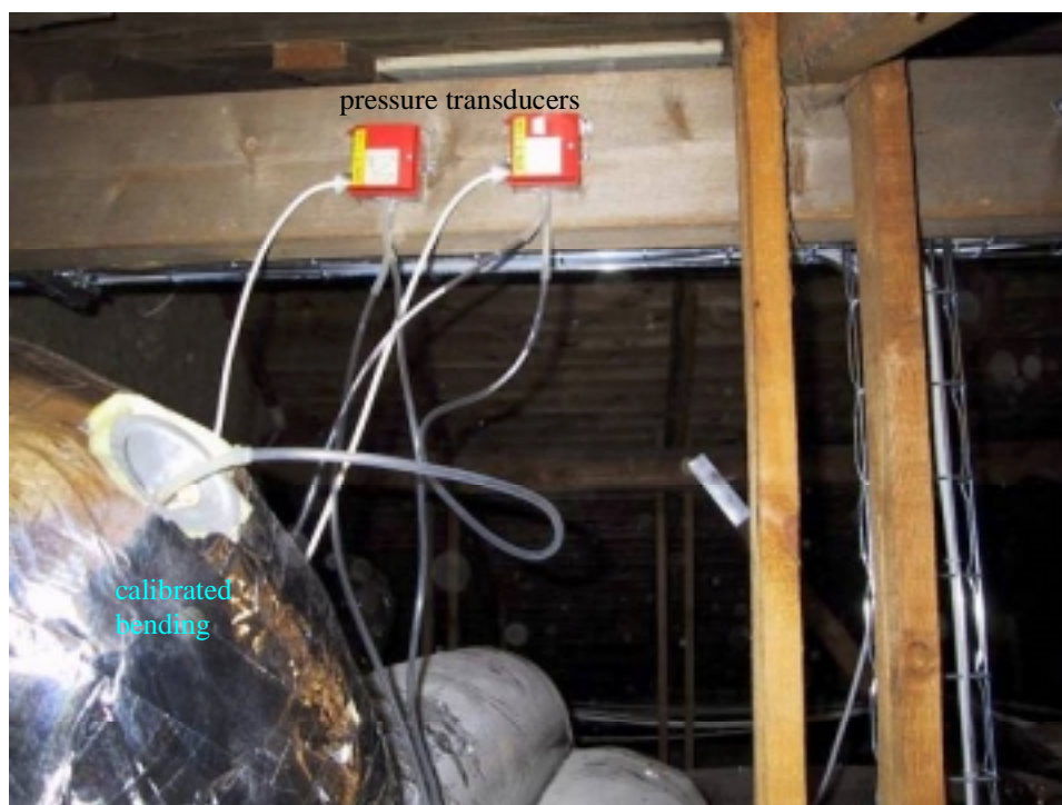
Figure 2.16. The applied pressure transducers for determination of the volume flow rates.
