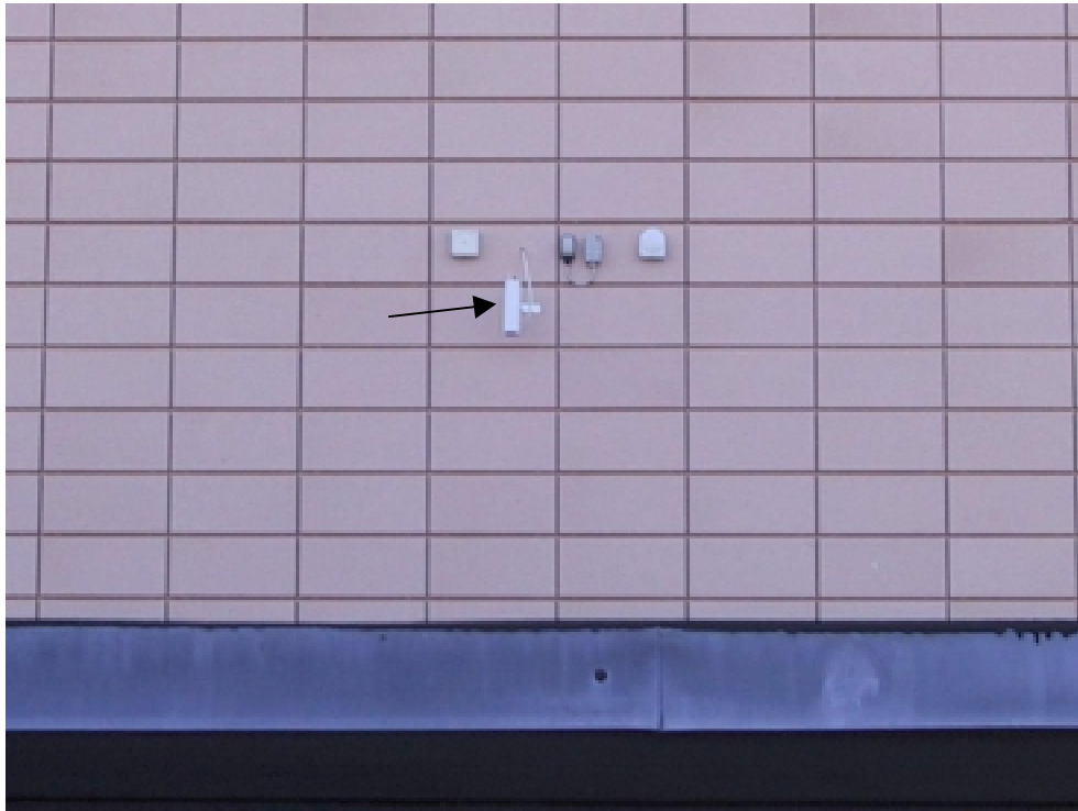
Figure 2.3. The double shielded ambient temperature sensor.
