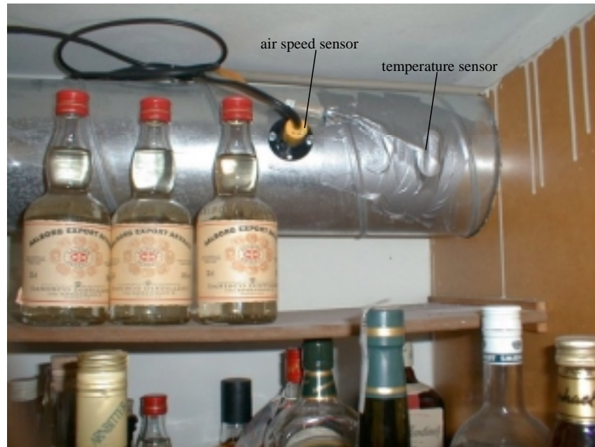
Figure 2.9. The air speed sensor and temperature sensor in the exhaust duct.
