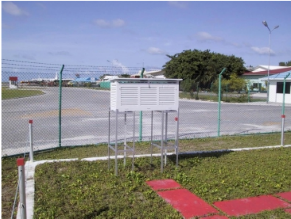
Figure 20. One of the English huts at the meteorological station for shielding the ambient temperature and relative humidity sensor.
