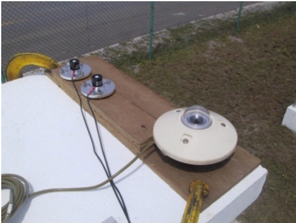
Figure 8. Set up for calibration of the pyranometers.
