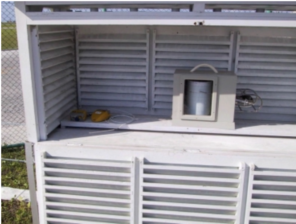
Figure 23. The two Tinytag data loggers located in one of the English huts of the meteorological station.
