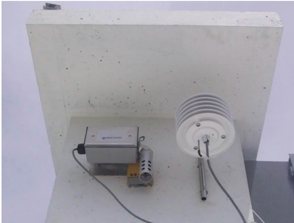
Figure 7. The shielded ambient temperature sensor (to the right) and the sensor for measuring relative humidity (to the left).
