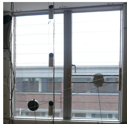
Figure 3 The view out of test room A with a low-e window with MicroShade.
