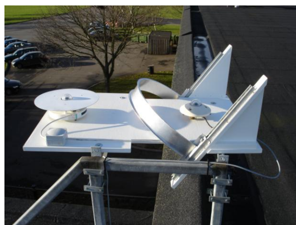
Figure 5 The solar measuring station.
